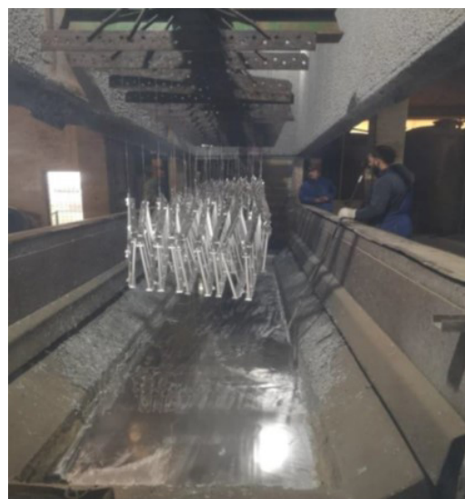
Fig.1 Retrieving parts from thermal galvanizing process
