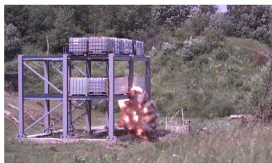
Fig. 2. Near field blast (FRAMEBLAST project, https://www.upt.ro/centre/cemsig/frameblast.htm )
