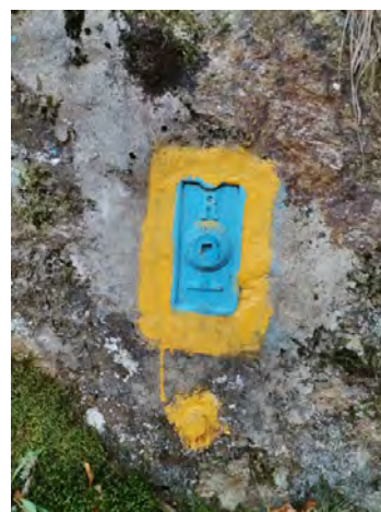
Leveling landmark, Breazova Dam, Caraș-Severin County
